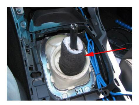
Step 8: Remove the foam padded surround from the shaft to reveal the bolts for the factory shaft mount.
