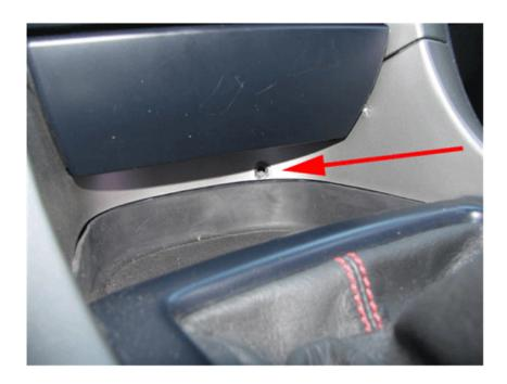
**Step 2**: Using a phillips head screwdriver, remove the single screw located under the headunit area in front of the gearshift.
