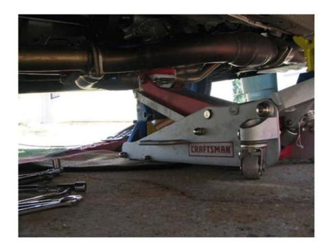
**Step 11**: Locate your jack under the gearbox, in order to support the weight of the box when loosening off the gearbox cross member bolts to aid in installation.
