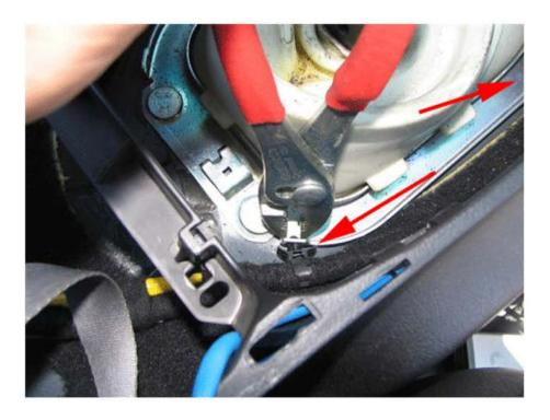
Step 10: Using pliers, carefully unclip the loom clips holding the wiring to the dust boot.
