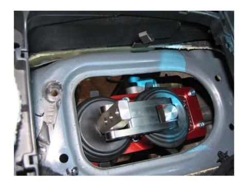
**Step 21**: Drop in your new Billet Pro series shifter, being careful not to move it around to much which may disperse the bead of sealant on the mating surface. Although not entirely necessary, its a good idea to use locktite on the mount bolt threads to to ensure secure fitment.
