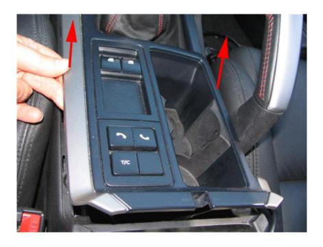
**Step 3**: As you pull the consolde section upwards, you will notice the sound of clips 'unclipping', this is normal, however do take care not to damage these by pulling too hard.
