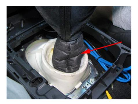
Step 26: Re-install foam shaft pad and connect up the clips for the factory boot surround.
