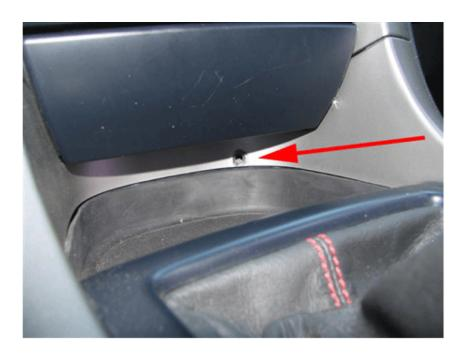
Step 28: Re-fit the front retaining screw for the console.
