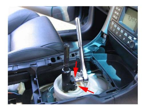
Step 9: Using a 10mm socket piece on a ratchet, undo the two bolts holding the shaft to the factory shifter.
