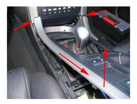
**Step5**: Now the console is free of obstruction, carefully lift the back section upwards to free the front section where it hooks up under the center dash as indicated by the arrows in the picture above. Place the console section aside where it wont be damaged.
