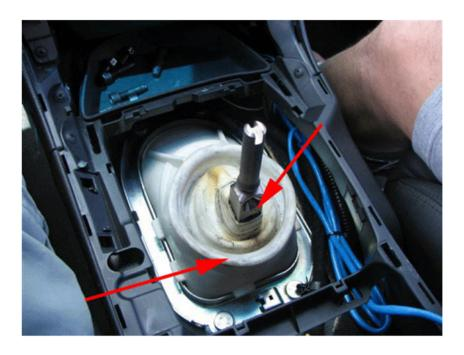
**Step 25**: You can now begin to re-assemble the interior parts. Starting with the white rubber dust boot. Remember the nuts for these on the underside of the vehicle.
