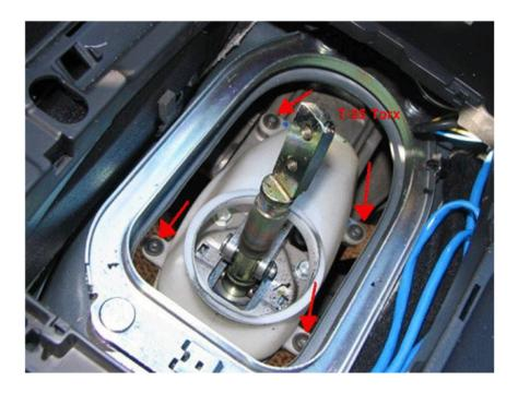
**Step 16**: Using a T25 torx driver, or a normal screw driver if accessible, remove the four screws holding the plastic dust cover.
