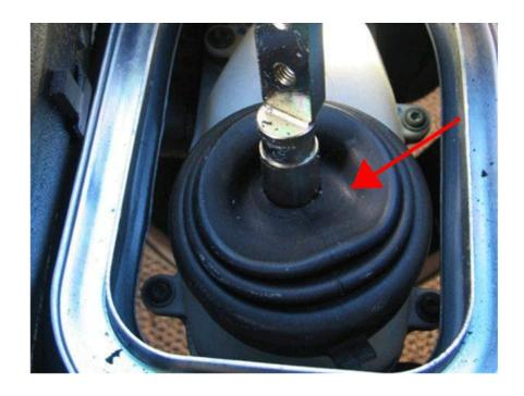
Step 15: Remove the factory black rubber dust cover. (no longer needed for installation)
