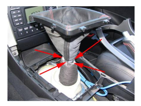
**Step 7**: Using a flathead screwdriver, carefully pry the clips away from the to unhook the boot from the shaft, then firmly holding the gear knob, pull upwards to remove the factory knob. Please note that he knob is glued from factory and takes some force to remove, be mindful not to injure yourself in the upward motion aside where it wont be damaged.
