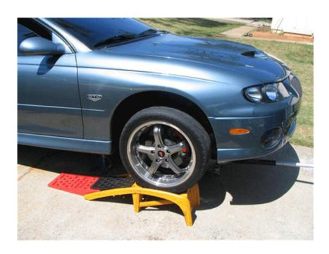
**Step 1**: With the gearbox in neutral, jack the vehicle up and support with jackstands under chassis rails, or alternatively drive your vehicle onto ramps. Safety is always the key, so please double check your jack stands and vehicle are on stable ground.
