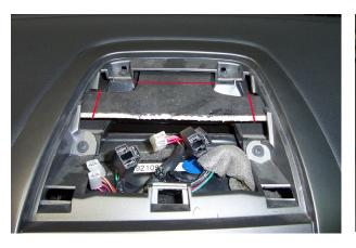
**13)** The other end of the wire harness should be pushed down through the opening as shown.
