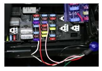
17) Plug the connector and the oil pressure sender 18) Clip the gauge in and peel the tape off. wire into the gauges as shown.
