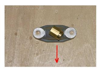
25) Screw the sensor into the connector.
