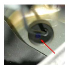
**21)** Route the wire under the coolant tank down along with the overflow hose.
