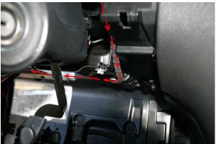
**15)** Attach the wires as shown on the picture. Black wire (ground) connects to the steering column bolt. It is highlighted blue on the picture. Connect the other three wires (white, red and pink) as shown on the picture insert: first, plug the wire into the right side of the fuse connector, then plug the fuse on top.
