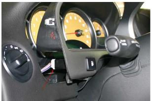
**8)** Unclip the fuse cover under the steering wheel by pulling it down.
