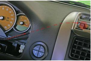
11) Cut along the red line. This allows for perfect fitment. NOTE: THIS MUST BE CUT OUT. IF YOU DON'T, YOU RISK DAMAGING THE COVER AND/OR THE GAUGE MOUNT POINTS WHEN YOU CLIP IT DOWN.
