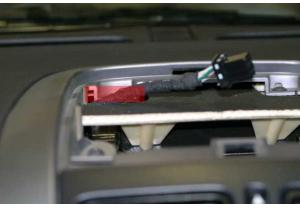
**14)** Route the wire underneath the steering column. You can use zip-ties to hold it in place at your discretion.
