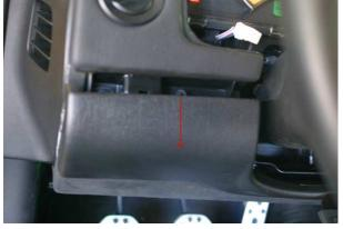
**10)** The connector of the wire harness should come out through the center of the dash as shown.
